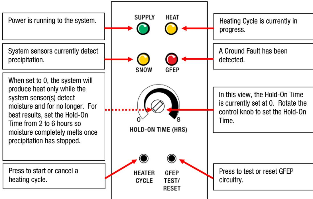
**Figure 6. GF Pro OPERATOR CONTROLS AND INDICATORS**
