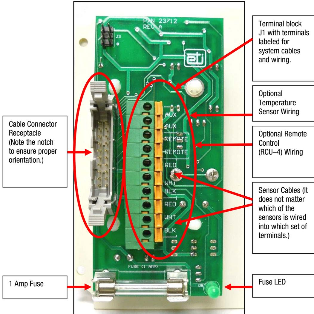
**Figure 4. THE GF Pro FRONT PANEL PC BOARD**
